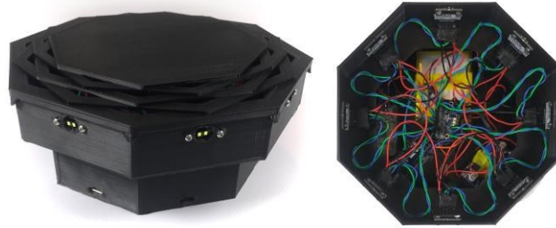
Figure 3. The inside and outside of the base station showing wiring and movement detection sensors on each side
