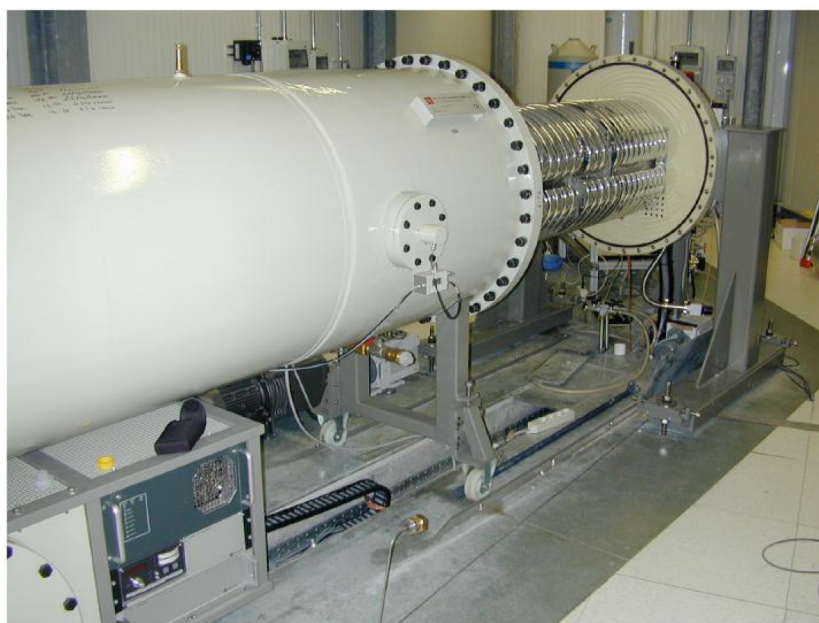
Figure 1. Open tank of the LUNA 400 kV accelerator. Inside the tank: the metallic rings keeping the ion source area free from electric fields, are visible.
