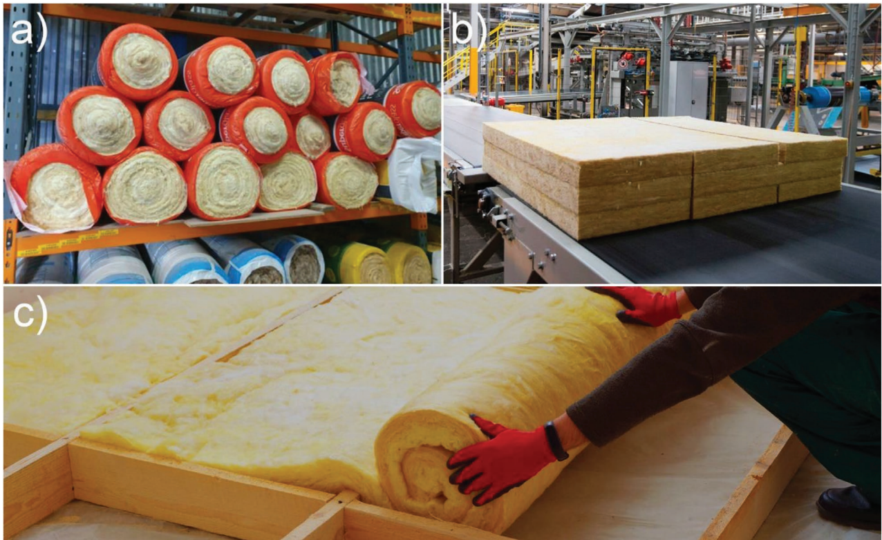
Figure 4. a) Packaged rolls of glass MWI. b) Cut slabs of glass MWI prior to packaging. c) An installer unrolling a MWI product at a construction site.
