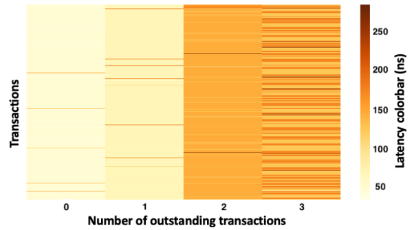
Fig. 2: Heat map showing the range and distribution of latencies for different DRAM loadings
