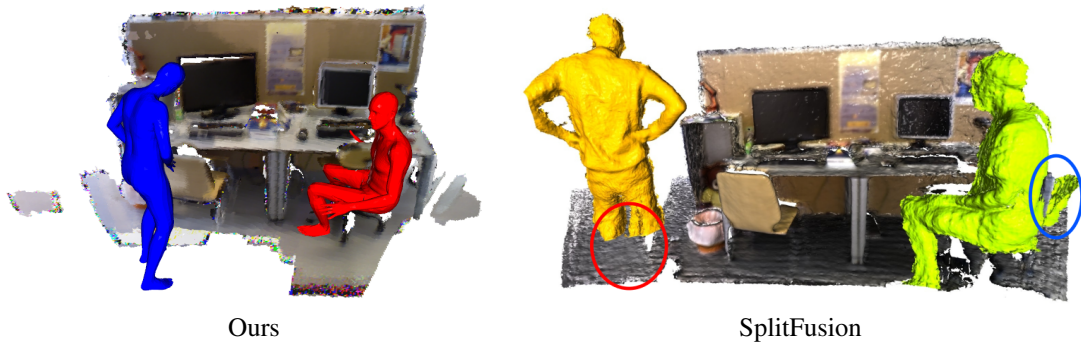
Fig. 5: Reconstruction results on fr3_walking_xyz sequence of TUM dataset. The input images are as same as Fig. 2. On the left, our method outputs complete and clear human meshes. On the right, SpF failed to track the fast subject (see missing feet circled in red). In addition, it cannot distinguish connected objects, e.g. , in the blue circle, the chair was fused into the green human mesh.
