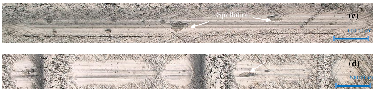
Figure7-14- DLC/1 coated Verogray substrate showing the deformation on (c) parallel (d) perpendicular orientation to the applied load of 1N.
