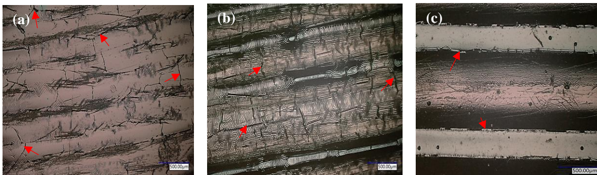
Figure 0-5- Cracking behaviour of DLC/5 coating on 3D ABS after bending showing coating deformation pattern on all three surfaces defined as (a) untextured coated surface (b) textured type A (c) textured type B.
