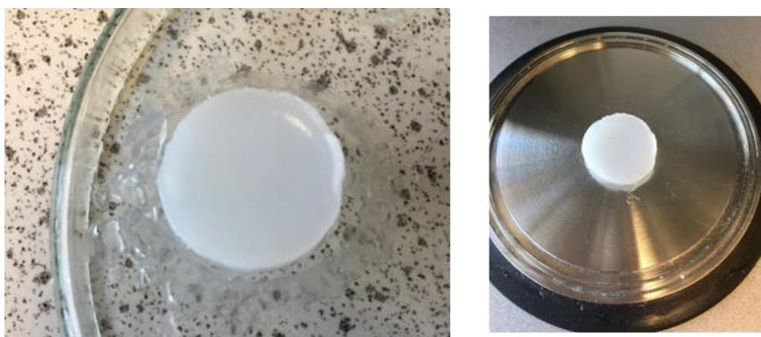
Figure 72. Gel samples for rheological studies. Left: The sample once the bottomless vial has been removed. Right: a sample once it has been transferred to the rheometer.
