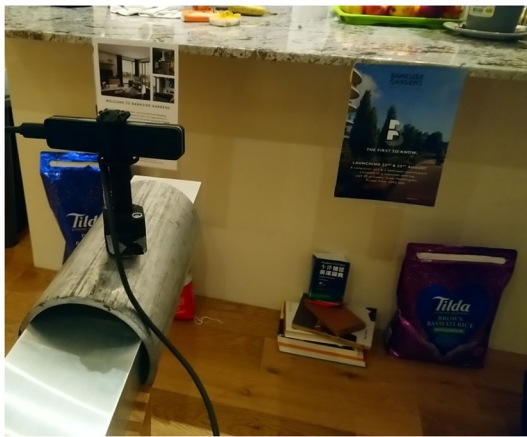
Fig. 5 Scene of the measurement including scanned sample, EMAT holder and attached zed camera and background that the zed camera is looking at
