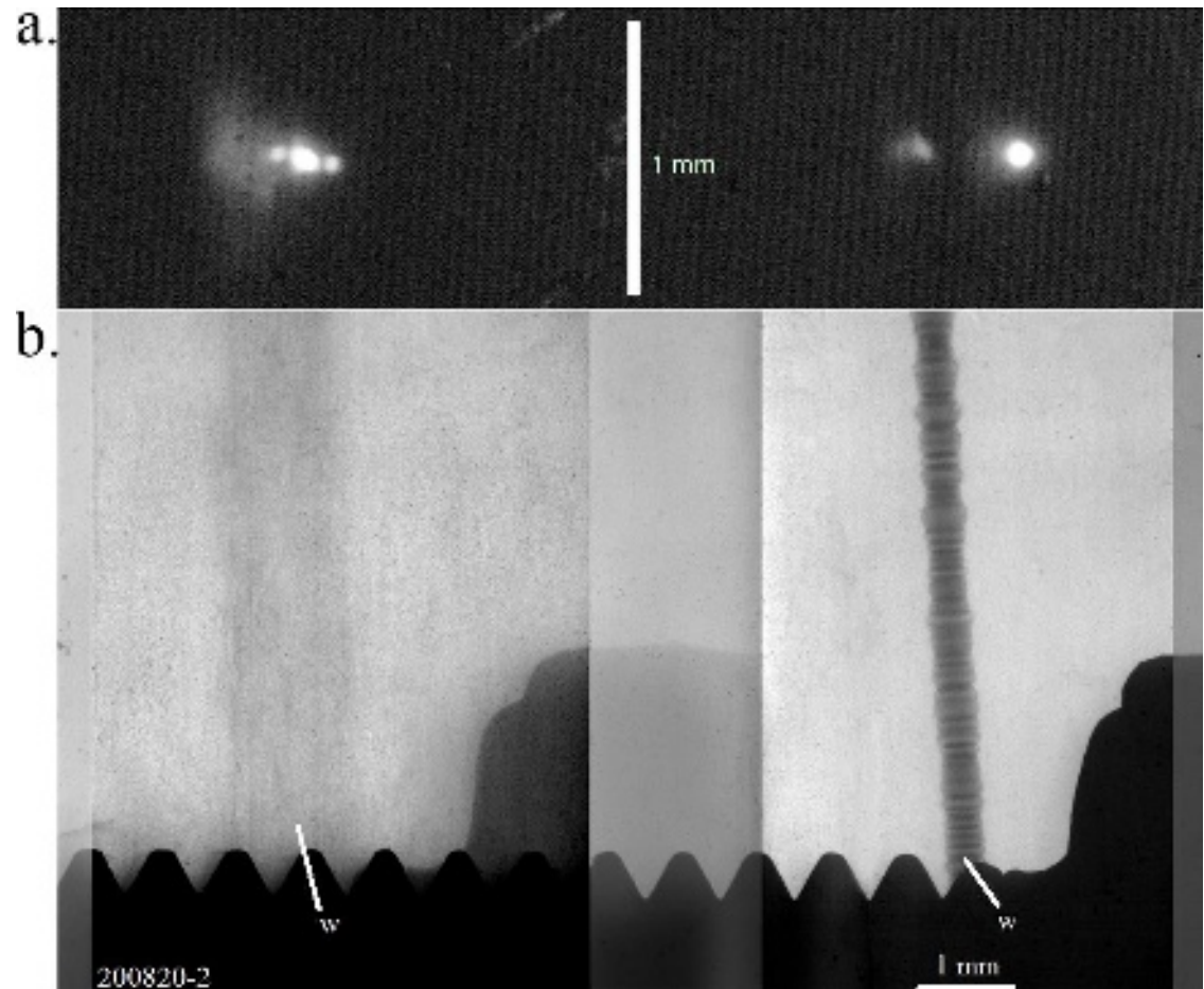
Fig.5. Pinhole image of the HXPs (a) and radiograph images (b) of the exploding 25 \mu\text{m} Ag wire in two moments of time: 90 ns (right) and 125 ns (left).
