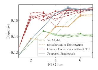
Fig. 2: Evolution of process cost with the RTO iterations. Circles represents the violation of a constraint.
