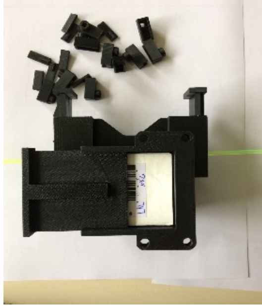
Figure 6. 3D printed external head for housing the external trigger assembly and the ^{22}\text{Na} source.
