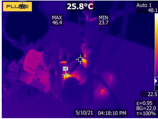
(b) Transistor temperature for \theta_B \simeq -60^\circ
