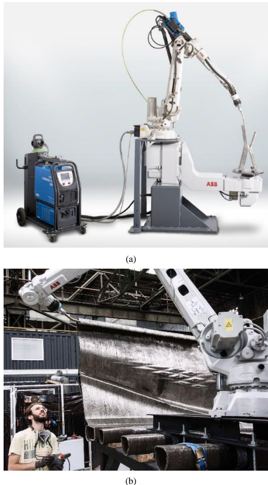
FIGURE 1. (a) WAAM robotic facility and (b) WAAM of the MX3D bridge
