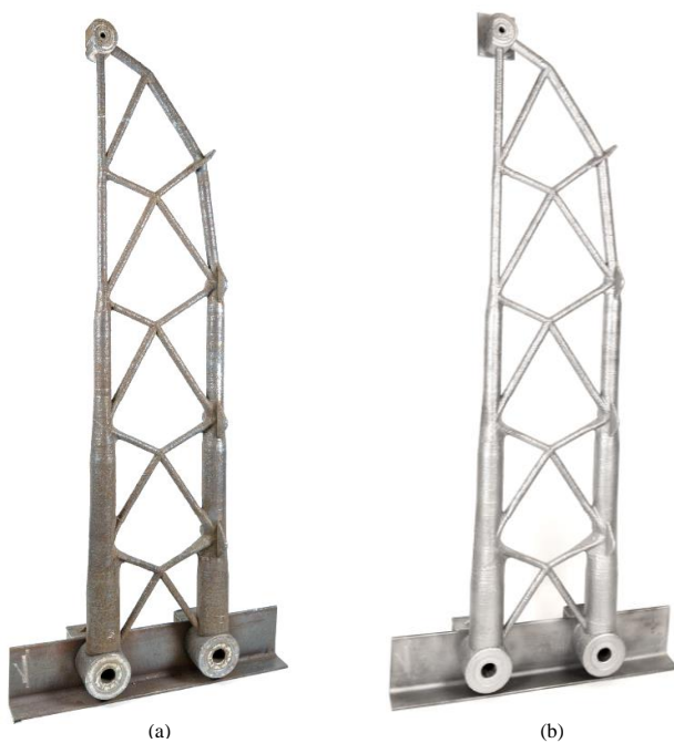
FIGURE 19. Cantilever truss (a) before and (b) after sandblasting
