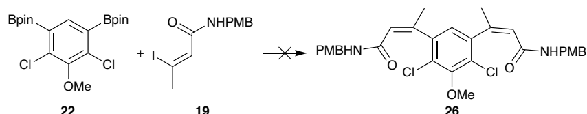
Scheme 10 – Failed reported literature coupling of 22 and 19 to form 26. For attempted reaction conditions see Appendix 7.1.3 Table 3.
