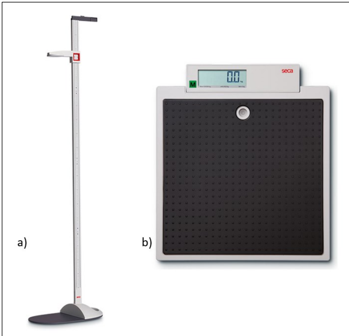
Figure 3.4. a) Leicester Height Stadiometer (Model 217, Seca, Hamburg, Germany); b) Seca Dual Measurement analogue scales (Model 761 Seca, Hamburg, Germany).
