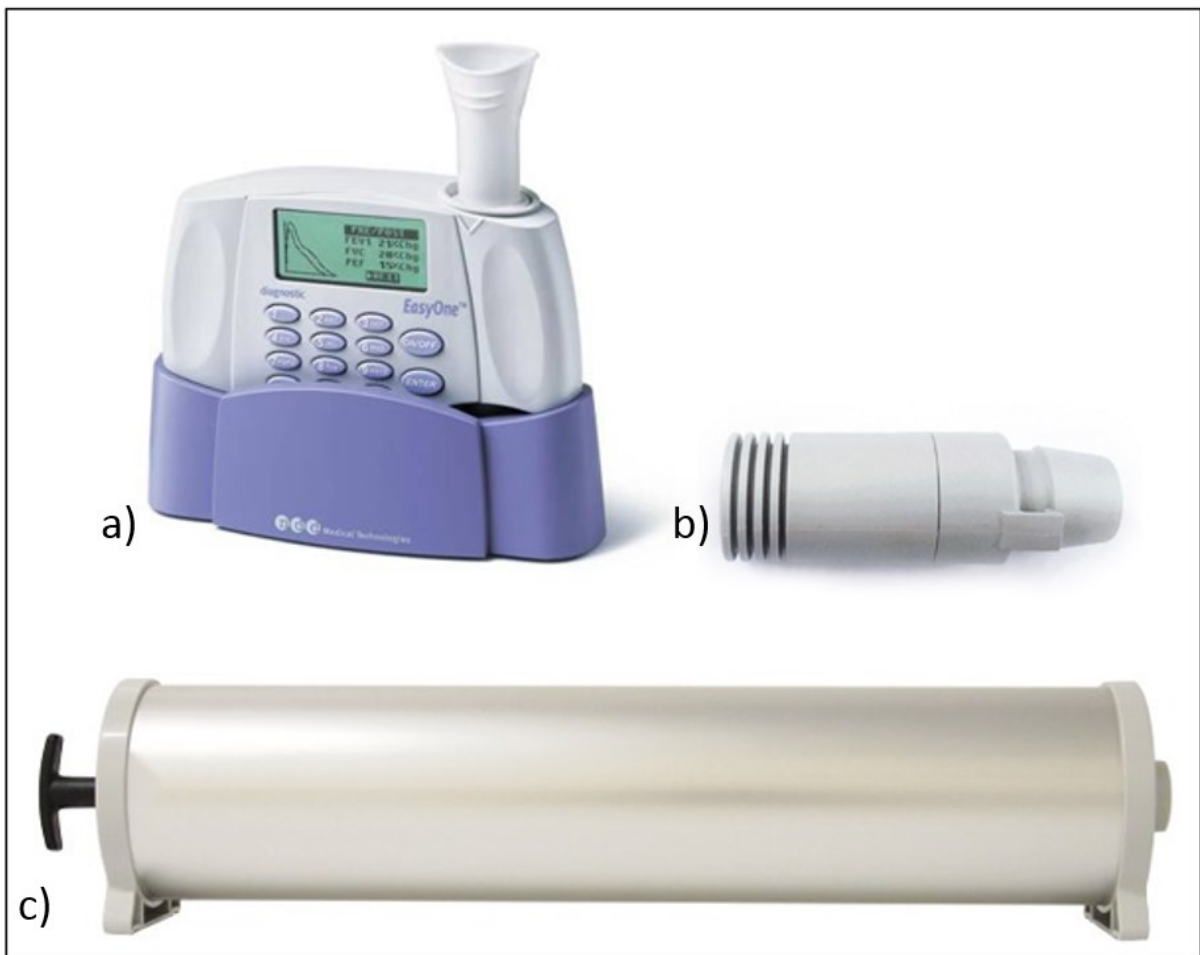
Figure 3.6. a) EasyOne diagnostic spirometer; b) Calibration adapter; c) 3-litre calibration syringe.
