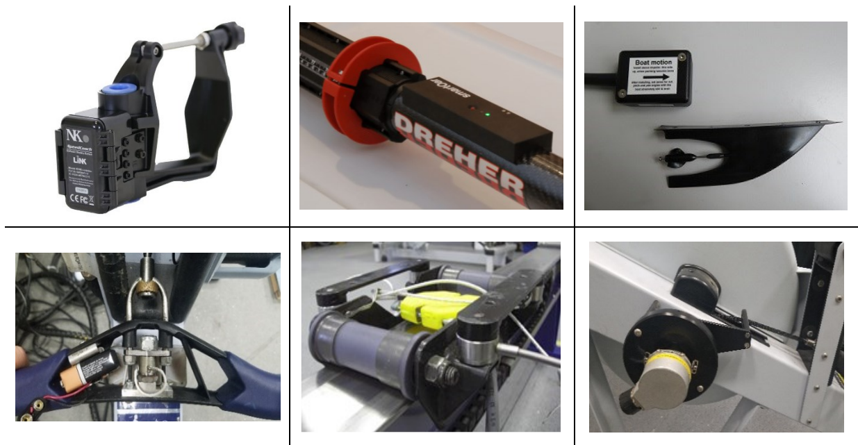
Figure 3.4: On-water and on-ergometer data acquisition systems. Clockwise from top left: oarlock gate angle sensor (Nielsen-Kellerman, 2017); oar shaft force sensor (SmartOar, 2016); boat hull impeller/velocity sensor (Nielsen-Kellerman, 2021); flywheel rotary displacement transducer; under seat force sensors; inline handle uniaxial load cell.
