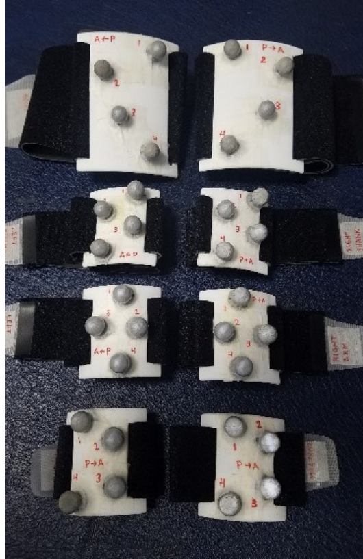
Figure 5.6: Custom 3D printed nylon rigid cluster plates with elastic Velcro bands for securing to body segments and four 14 mm retroreflective markers affixed per plate.
