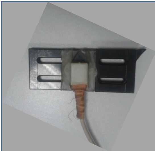
Figure 4.2: Electromagnetic (EM) sensor, FoB3, affixed to plate with stylus tip ( left ). EM sensor, FoB4, affixed to anterior tibia plate ( right ).
