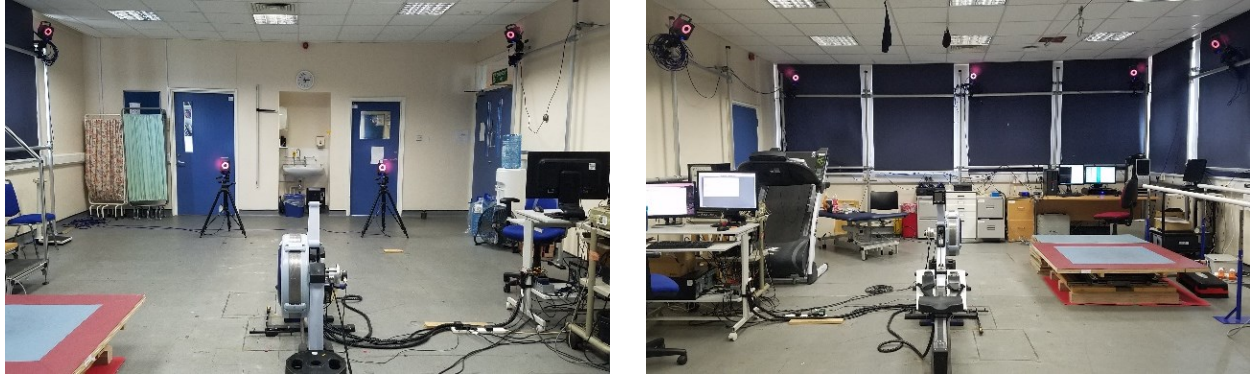
Figure 5.4: Biodynamics laboratory with modified ergometer at the center of the room surrounded by ten Vicon MX-T infrared cameras.
