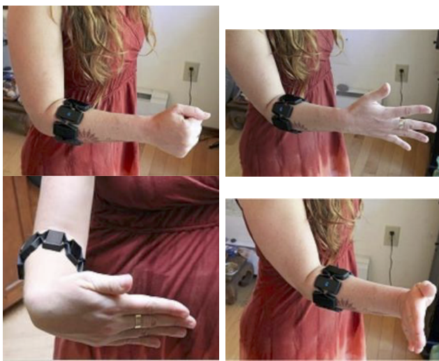
Fig. 2. Gestures used for familiarisation with Myo. Left to right: Closed fist, fingers spread, wrist flexed and wrist extended
