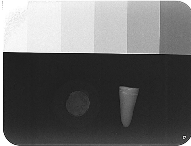
Figure 21: Radiopacity of HA printed root and HA disc compared with the aluminium step wedge. The radiopacity of HA printed root and the HA disc was approximately equivalent to 2 and 1 mm of aluminium thickness, respectively
