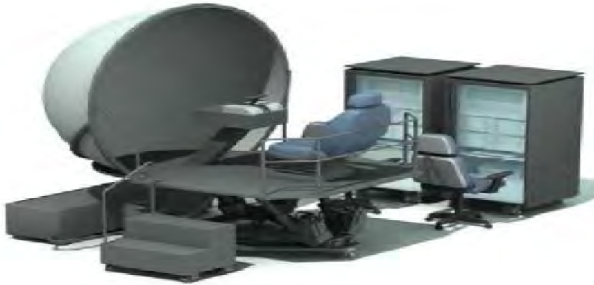
Figure 22: Graphical rendering of a tilting train simulator. Source (Kwangsoo et al.)
