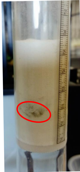
Fig. 2.3. A large void, visible, at the side of a fluidised bed, of 0.03 m dia. The void, highlighted in red, is caused by a large, submerged sphere which has come to equilibrium beneath the surface of the bed.
