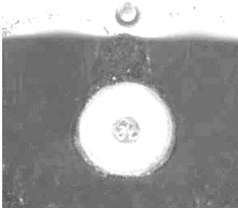
Fig 3.3. A 12 mm diameter cylinder, viewed from the end, in a 2-D bed of incipiently fluidised particles at room temperature. The image is a time-averaged image of 10 s recording. The bed is blurred around the cylinder; however, above the cylinder a region of stationary particles can be seen. The image indicates there could be localised variations in density in the bed material.
