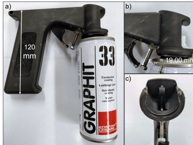
Fig. C.2 An outline of the modified spray can gun: a) side view of gun attached to the graphite spray can, b) close-up side view of the spray can gun showing the exposed bolt distance ( x_{spr} ) which controls the maximum trigger movement and thus the spray flow rate, and c) close-up front view of the spray can gun showing how the bolt limits the trigger movement.
