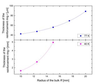
**Figure 10.** Minimum thickness of the ring reinforcement r required to provide compression at the centre of an Ag-containing Gd-Ba-Cu-O bulk of height D = 25 mm for the entire magnetisation process for several radii R (10 mm - 20 mm), as well as different temperatures T = [40 K; 77 K].
