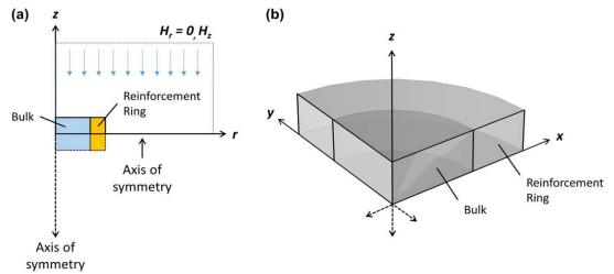
**Figure 1.** (a) Setup of a 2D axisymmetric numerical model of a (RE)BCO bulk with a reinforcement ring and an applied magnetic field in the z-direction in the r-z- $\varphi$  cylindrical coordinate system, as evaluated in [4]. (b) The equivalent 3D model [4]. © IOP Publishing. Reproduced by permission of IOP Publishing from [4]. All rights reserved.
