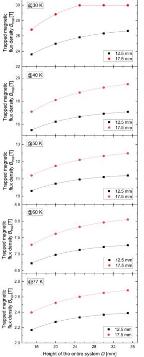
**Figure 13:** Trapped field at the end of the FCM process of an Ag-containing Gd-Ba-Cu-O bulk of radii R = [12.5 mm; 17.5 mm] reinforced by a ring of thickness r = 3 mm for several heights D (15 mm - 35 mm), as well as different temperatures (30 K - 77 K).
