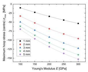
**Figure 16:** Maximum hoop stress at the centre of an Ag-containing Gd-Ba-Cu-O bulk of radius R = 12.5 mm and height D = 25 mm reinforced by a ring of thickness r (0 mm - 5 mm) and Poisson's ratio v = 0.3 for several values of Young's modulus E (100 GPa - 300 GPa) of the ring material at 60 K.
