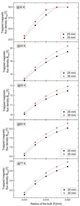
**Figure 14:** Trapped field at the end of the FCM process of an Ag-containing Gd-Ba-Cu-O bulk of heights D = [25 mm; 35 mm] reinforced by a ring of thickness r = 3 mm for several radii R (15 mm - 35 mm), as well as different temperatures (30 K - 77 K).
