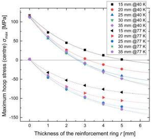
**Figure 11.** Maximum hoop stress at the centre of an Ag-containing Gd-Ba-Cu-O bulk of radius R = 12.5 mm reinforced by a ring of thicknesses r (0 mm - 5 mm) for several bulk heights D (15 mm - 35 mm), as well as different temperatures T = [40 K; 77 K].
