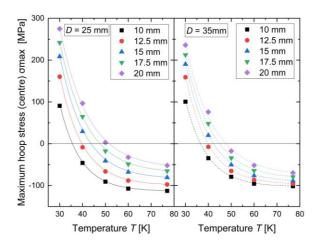
**Figure 7.** Maximum hoop stress at the centre of Ag-containing Gd-Ba-Cu-O bulk of heights D = [25 mm; 35 mm] reinforced by a ring of thickness r = 3 mm for radii R (10 mm - 20 mm), as well as different temperatures (30 K - 77 K).
