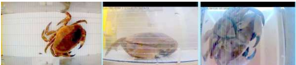
Figure 12 Chute 2 camera views showing (from left to right) the measurement camera view, the off-set camera view and the sex determination camera view.
