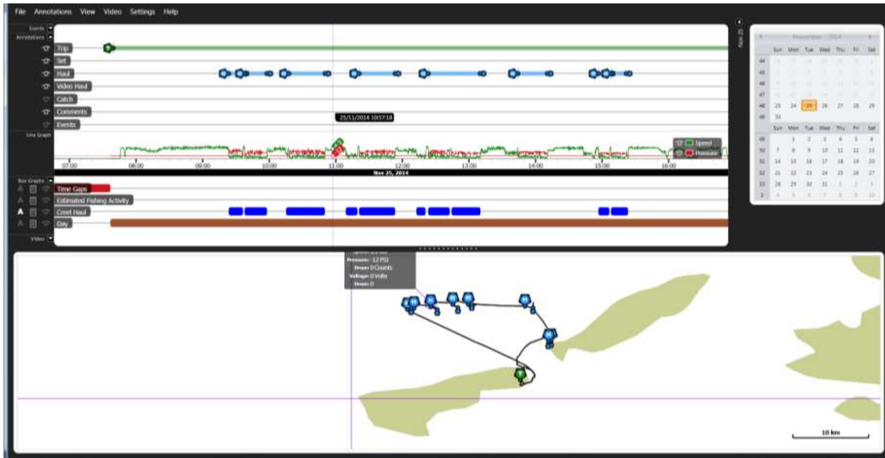
Figure 3.5 A completed annotation file for the same data set but with only 1 trip selected for display. Note the speed and hydraulic pressure readings on the line graph which are used to identify string hauling position.
