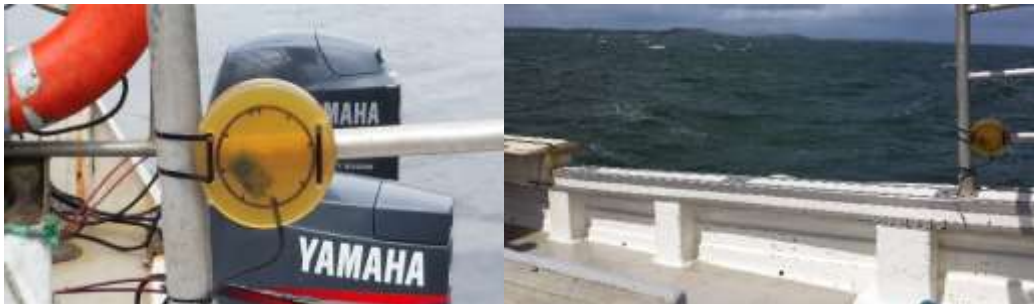
Figure 4.1 The AMR designed RFID readers. A close up view of the shooting reader (left) and a view of both readers (right), with the haul reader just visible on the left side of the gunwale.
