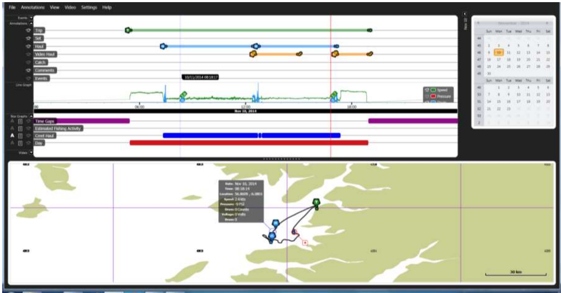
Figure 3.6 A completed annotation file for one trip on a towed gear vessel. Note the blue line graph reading showing winch rotation activity. Also shown is the actual footage reviewed by the video analyst (orange).
