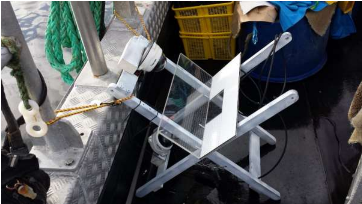
Figure 4.9 Chute 1 in-situ on fishing vessel.
