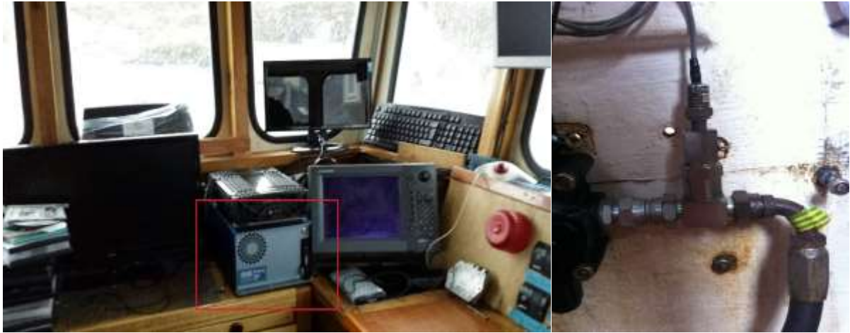
Figure 1.3 An Archipelago Marine Research EM Record v4.5 control box and a hydraulic sensor.
