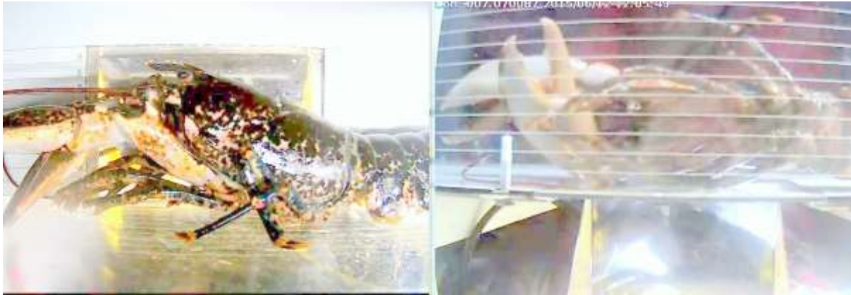
Figure 4.10 The 2 camera views required to determine carapace length from 1st chute design, Image of lobster against calibrated surface (left) and view of underside (right) to determine sex and off-set (distance above calibrated measuring platform).
