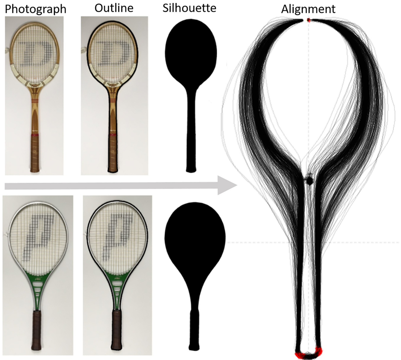
Fig 1. Image processing examples for shape analysis. All rackets were photographed from above. Matlab was used to make an outline and fill for a silhouette image. All silhouette images were then inputted to the R Package Momocs and aligned via a Procrustes alignment on three coordinates (red points). All photographs of the rackets were taken by the authors.
