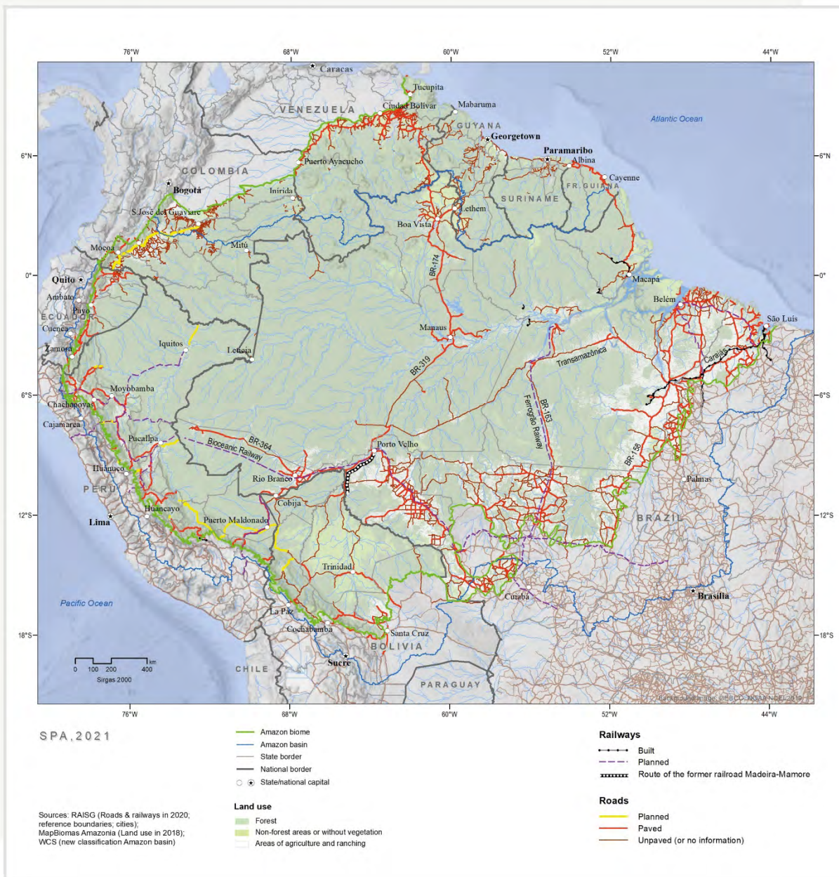
Figure 19.6 Planned (yellow), paved (red), and unpaved (brown) roads across the Amazon, as well as existing (black) and planned (purple) railways. The Amazon biome is outlined in green, while the Amazon Basin (the limit used in other chapters of this report) is outlined in blue.
