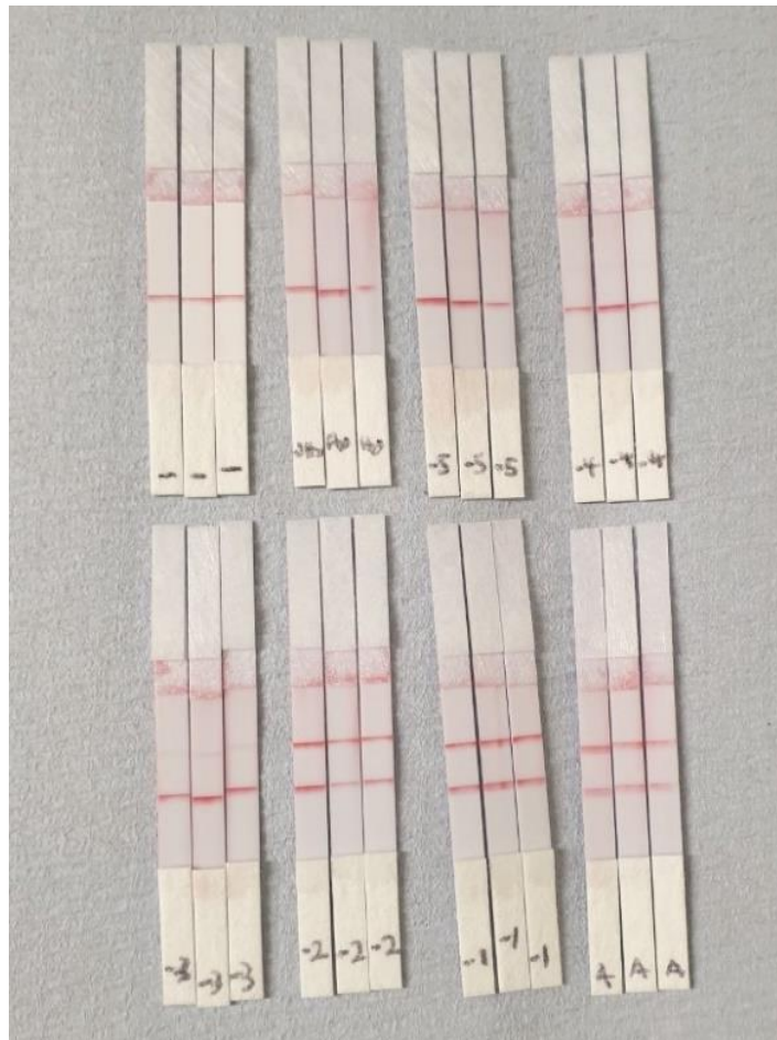
Figure 2-13: Effect of dilution of LAMP amplicons on LF read-out. LAMP was conducted using the qPCR machine, the amplified samples were serially diluted and added to the LF strips with two drops of Wash Buffer (supplied with the strips). The LF strips are marked with their respective sample, Water (-), LAMP negative control ( \text{H}_2\text{O} ), serially diluted amplified samples: 100,000X dilution (-5), 10,000X (-4), 1,000X (-3), 100X (-2), 10X (-1) and A is the original amplified solution.
