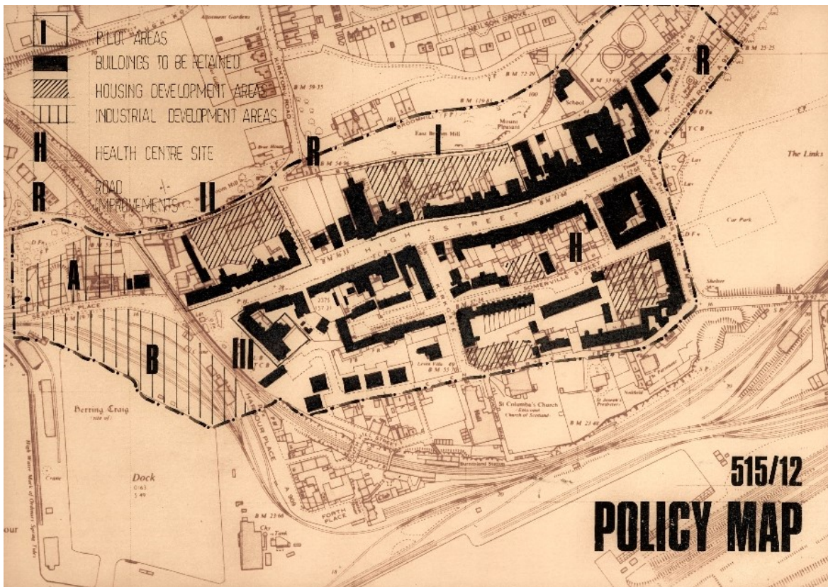
Figure 6.3. Wheeler & Sproson's Policy Map of Burntisland, indicating features such as areas for future housing, buildings to be retained and industrial development areas.
