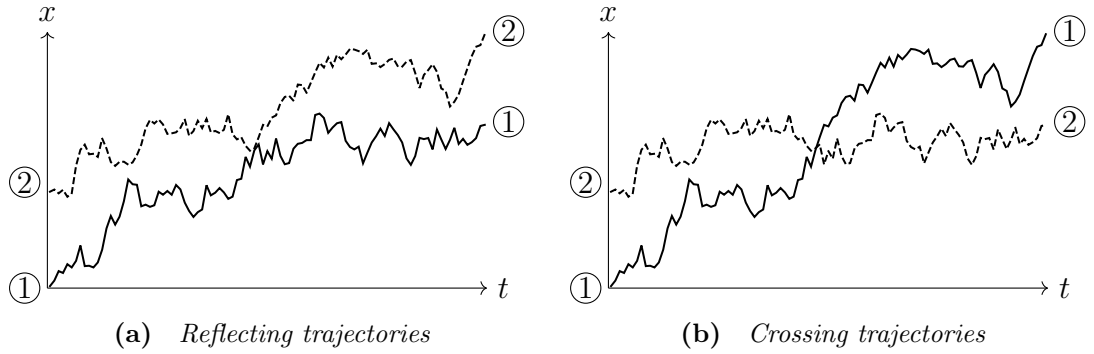
Figure 3.2 Two non-interacting identical Brownian particles cannot be distinguished at a point of crossing. The left and right scenario therefore have identical probability.
