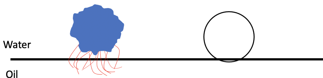
Figure 5.22: Schematic of the SZ adsorption mechanism showing the comparison to a spherical particle (right) and microgel (left). For the microgel the blue represents the hydrophilic sections and the red being the hydrophobic chains which mediate adsorption to the interface.
