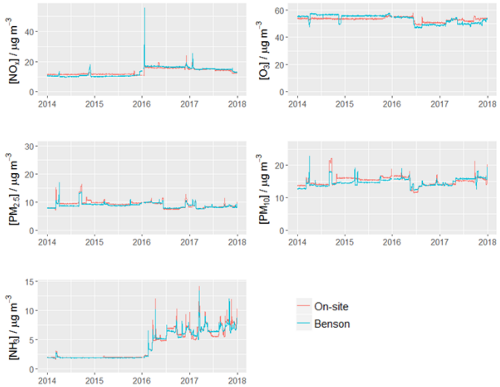
Figure S3: Comparison between deweather model (Carslaw, 2015) outputs of predicted concentrations of \text{NO}_x , \text{O}_3 , \text{PM}_{2.5} , \text{PM}_{10} and \text{NH}_3 for different sources of meteorological data. Shown in blue are predicted deweather concentrations using measurements of wind speed, wind direction, air temperature, relative humidity and pressure from Benson (2014-2017). Shown in red are the concentrations using the same methodology but with a concatenated time series of the meteorological parameters measured on-site at Harwell (2014-15) and Chilbolton (2016-17).
