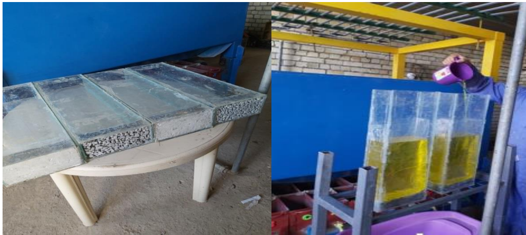
Figure 12: Permeability measurement of porous concrete
