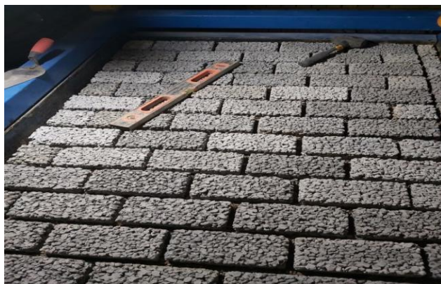
Figure (4): Porous interlocking pavement and layer (PICP) filter
