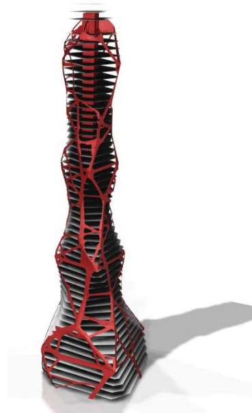
Figure (16): Results of a topology optimization study considering the exterior of the Bionic Tower as the designable domain
