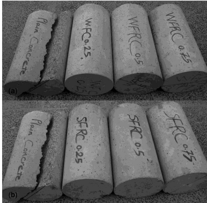
Figure 4: Comparison of failure pattern of FRC specimens after splitting tensile strength: (a) WFRC; (b) SFRC
