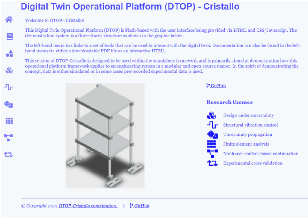
Figure 3. Landing page of DTOP-Cristallo showing the available simulations and a CAD model of the three-storey structure.
