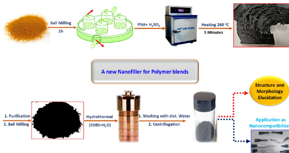
Figure 1. Schematic flowchart of PNA-based foam production, nanomaterial extraction, and their application as a nanofiller in the composites.
