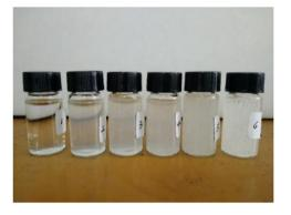
Fig. 5. Gel-type SPW solutions stored in bottles after 7 days.
