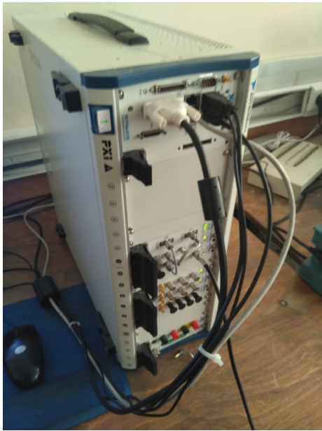
Fig. 2: The used digital oscilloscope type PXI-5114
