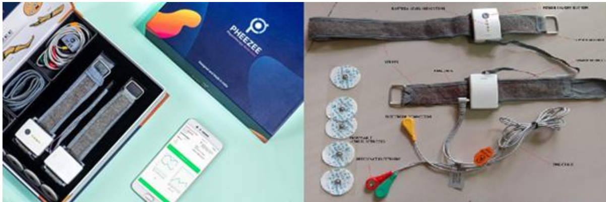
Fig-1: Pheeze toolkit with its parts and as a package the supporting phone app.
