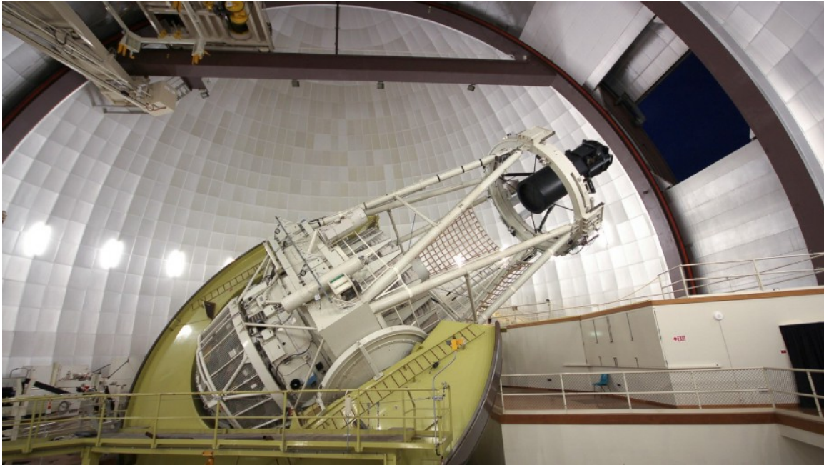
Figure 1.13. The Anglo-Australian Telescope (AAT) in suburban Sydney. Attached is the SAMI IFU instrument, used observe nearby galaxies as part of the SAMI survey. Image credit: AAO.
