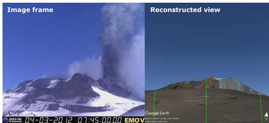
Fig. 4.3 An example of how the field of view (horizontal) was calculated by determining the left and right margins of the image frame (left and right green lines) on Google Earth.
