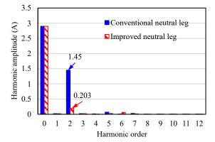
Fig. 19. FFT analysis of  $I_{dc}$ .
