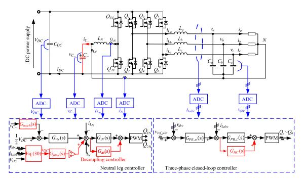
Fig. 6. Control for the improved neutral leg and the three-phase inverter.
