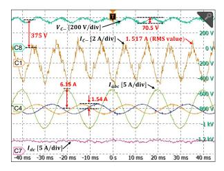
Fig. 25. Capacitor current waveform (C1) of the improved neutral leg.
