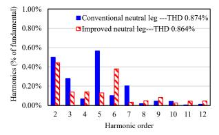
Fig. 20. FFT analysis of load voltage  $V_a$ .
