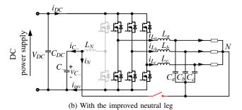
Fig. 28. Three-phase four-wire inverter with neutral legs in open-circuit failure mode.
