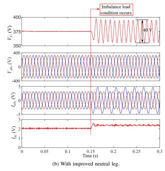
Fig. 13. Simulation results of inverters with conventional and improved neutral legs.
