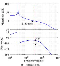
Fig. 12. Bode plots of the three-phase inverter.
