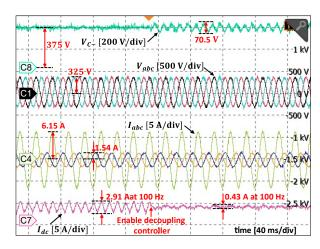
Fig. 21. Transient response of the decoupling controller in the improved neutral leg.
