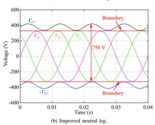
Fig. 14. Verification of capacitance requirement in Simulation.
