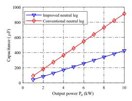
Fig. 4. Comparison of total dc capacitance ( $V_{max}=750~\mathrm{V}$ , imbalance factor  $\delta=0.5$ ).
