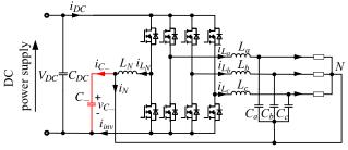
(b) With the improved neutral leg by removing  $C_{+}$ .
