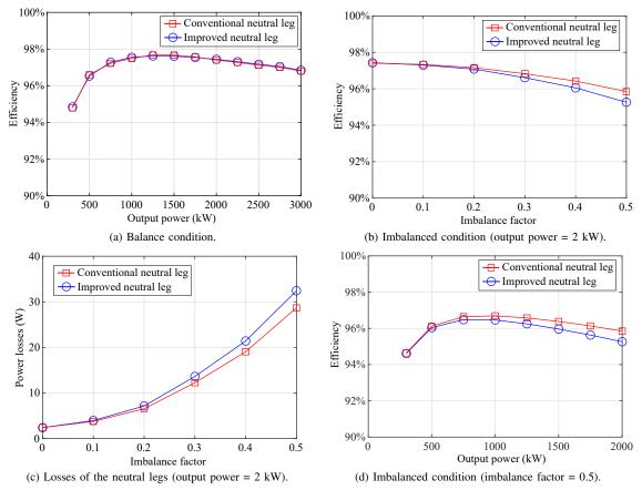
Fig. 23. Efficiency of three-phase four-wire inverters with conventional and improved neutral legs.
