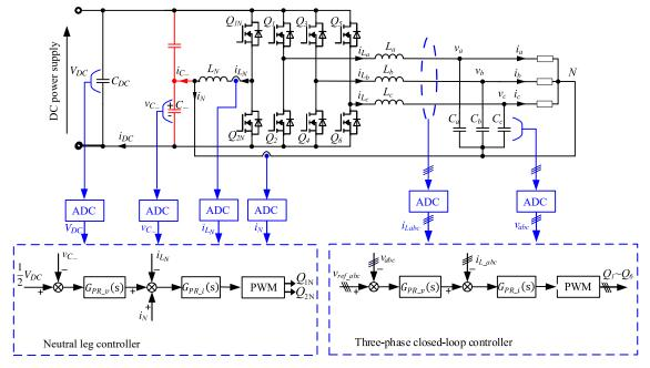
Fig. 7. Control for the improved neutral leg and the three-phase inverter.
