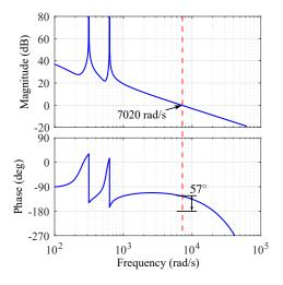
Fig. 9. Bode plot of the current loop for the improved neutral leg.
