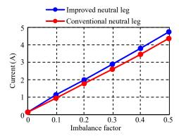
Fig. 24. Current stress of the neutral legs (output power = 2 kW).
