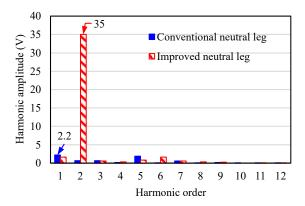
Fig. 18. FFT analysis of capacitor voltage  $V_{C_-}$ .
