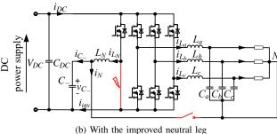
Fig. 27. Three-phase four-wire inverter with neutral legs in short-circuit failure mode (lower switch).
