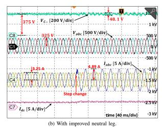
Fig. 22. Transient response of inverters with conventional and improved neutral legs in experiment. Step load change from balance condition ( $R_a=R_b=R_c=105\,\Omega$ ) to imbalance condition ( $R_a=R_b=105\,\Omega$ ,  $R_c=70\,\Omega$ ).
