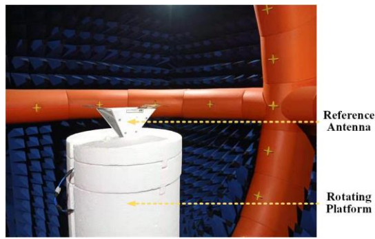
Fig. 13. Antenna radiation pattern measurement environment in a multi-probe AC.
