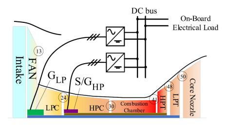
Figure 1.8: Concept diagram of the dual-channel power generation system [18].
