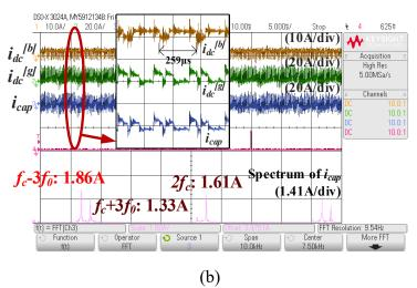
Figure 7.19: Harmonic suppression when  $P^{[g]}=1kW$ ,  $P^{[b]}=0.5kW$ . a) Without suppression. b) With EGW suppression.
