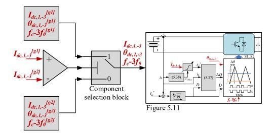
Figure 6.3: Modified local controller of the DC-DC converter.
