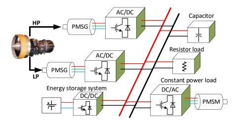
Figure 1.6: "Single bus" EPS structure.
