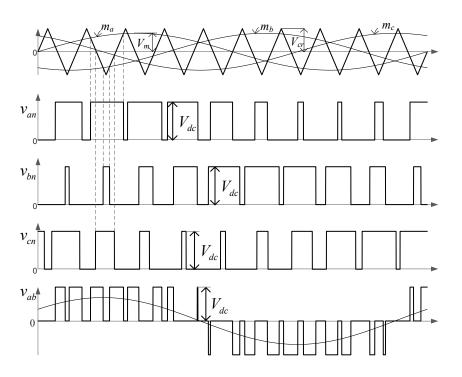
Figure 2.4: Sinusoidal pulse-width modulation (SPWM).
