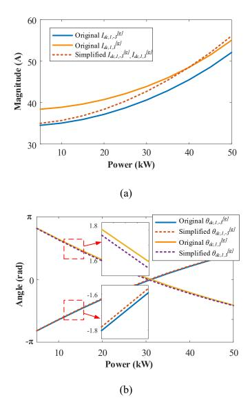
Figure 5.2: Comparison between magnitudes of the simplified and original model on  $f_c$ -3 $f_0$  and  $f_c$ +3 $f_0$ . a) Magnitudes. b) Angles.
