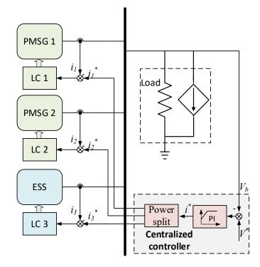
ratio of sources [28][96]. The algorithm of splitting current reference can be average splitting [28][96] or unequal splitting [97].
