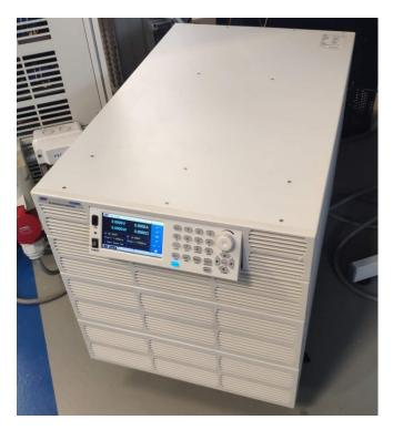
Figure 7.8: Programmable DC electronic load (EL600VDC19800W)
