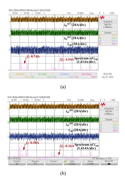
Figure 7.17: DC-bus and capacitor current when output power is 4kW. a) Without phase shift. b) With optimised phase shift angle (93°).
