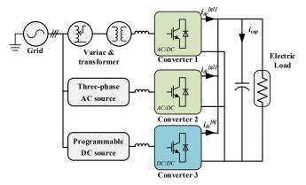
Figure 7.23: Experiment diagram.
