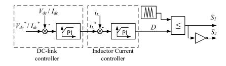
Figure 2.10: Controller of the DC-DC converter.
