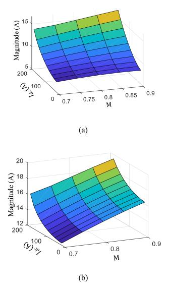
Figure 3.10: Magnitudes of first band harmonics related to the modulation and dc-link current. a)  $f_c$ -3 $f_0$ , b)  $f_c$ +3 $f_0$ .
