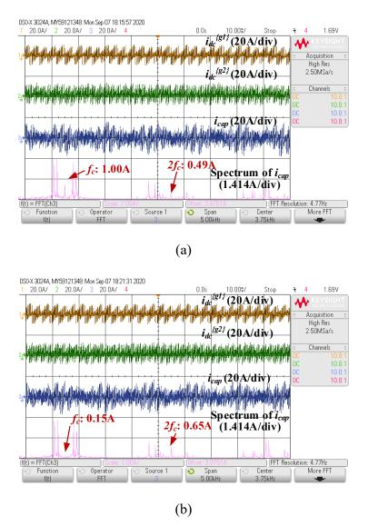
Figure 7.16: DC-bus and capacitor current when output power is 400W. a) Without phase shift. b) With an optimised phase shift angle (180°).
