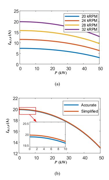
Figure 4.3: Magnitude of first switching harmonic. a) Magnitudes under different rotor speeds, b) Comparison between simplified model (4.22) and accurate model (4.10) when rotor speed is 32kRPM.
