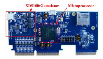
Figure 7.2: Texas Instruments F28379D controlCARD.
