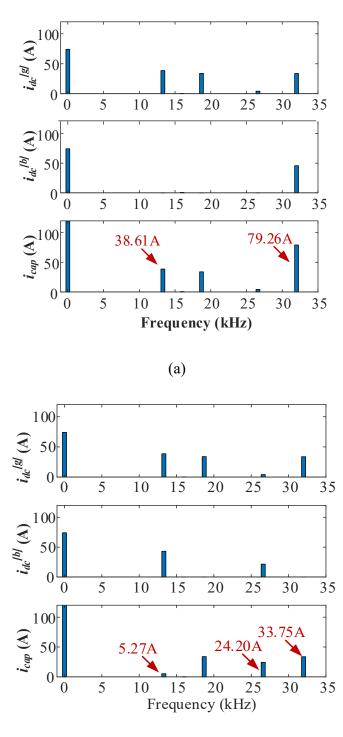
harmonics on  $f_c$  and  $2f_c$ . These components are summed up together on the DC-link capacitor current.
