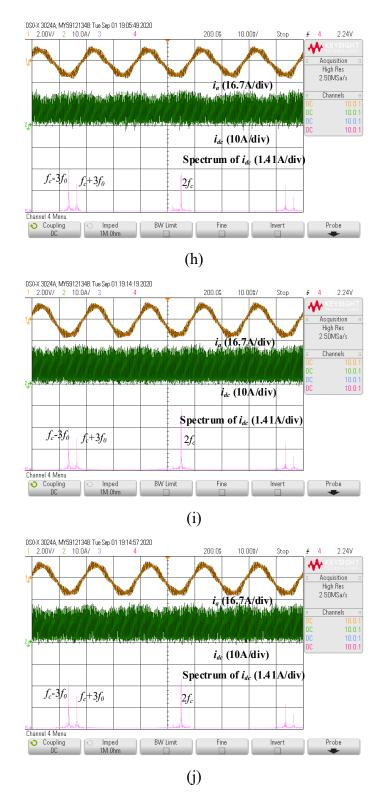
Figure 7.9: Phase current, DC bus current and its spectrum under different power (*P*) and modulation index (*M*). a) *P*=400W, M=0.9. b) *P*=400W, M=0.95. c) *P*=800W, M=0.9. d) *P*=800W, M=0.95. e) *P*=1200W, M=0.9. f) *P*=1200W, M=0.95. g) *P*=1600W, M=0.9. h) *P*=1600W, M=0.95. i) *P*=2000W, M=0.95. j) *P*=2000W, M=0.95.
