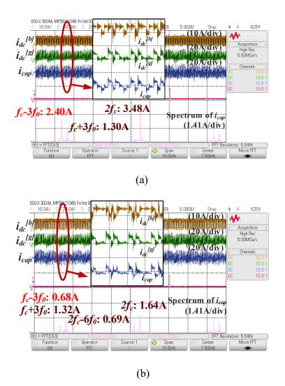
Figure 7.20: Harmonic suppression with EGW suppression when  $P^{[g]}=1kW$ ,  $P^{[b]}=1kW$ . a) Without suppression. b) With EGW suppression.
