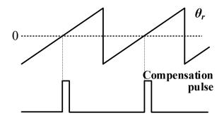
Figure 5.15: Compensation pulse generation.
