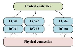
Figure 2.11: Operation principle of centralised control
