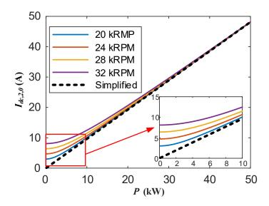
Figure 4.5: Comparison of second carrier harmonic component from accurate (4.24) and simplified (4.29) models with increased generator power and speed.
