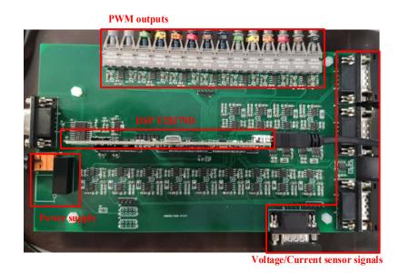
Figure 7.3: DSP Interface board.
