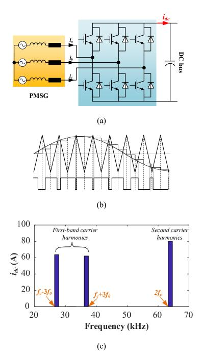
Figure 3.2: Two-level three-phase converter. a) PMSG and two-level converter, b) asymmetric regular sampling PWM, c) spectrum of  $i_{dc}$  (switching frequency  $f_c=32$ kHz, fundamental frequency  $f_0=1.5$ kHz).
