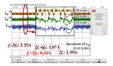
Figure 7.22: Harmonic suppression on  $f_c+3f_0$  with EGW suppression when  $P^{[g]}=1$ kW,  $P^{[b]}=1$ kW.
