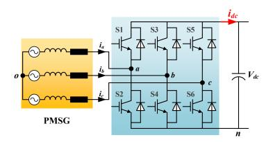
Figure 2.3: PMSG and two-level AC-DC converter.
