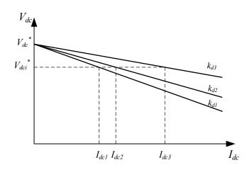
Figure 2.17: Power sharing characters of V-I droop control curve.
