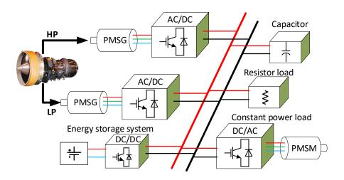
Figure 6.1: Typical dual-generation power system
