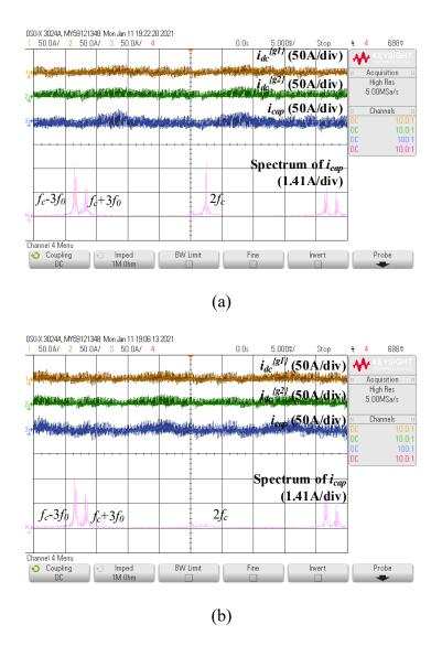
Figure 7.12: DC-bus and capacitor current when power sharing ratio is 1:1. a) Without phase shift. b) With 90-degree phase shift.
