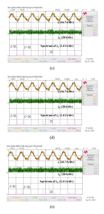
Figure 7.14: Phase current, DC bus current and its spectrum under different power (P) and fixed modulation index (M=1.04). a) P=400W. b) P=800W. c) P=1200W. d) P=1600W. e) P=2000W.
