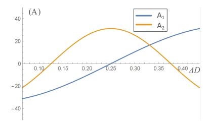
Figure 5.8: Magnitudes of the first and second carrier harmonic with  $\Delta D$  changing  $(f_c^{[b]} \text{ and } 2f_c^{[b]})$ .
