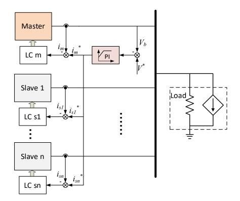
Figure 2.13: Control scheme of master-slave control.
