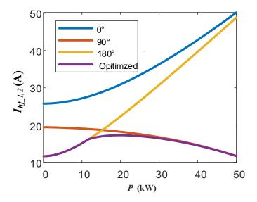
Figure 4.9: *I*<sub>*hf*\_1,2</sub> versus output power of single converter.
