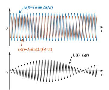
Figure 5.13: Sum up of two un-synchronised components.
