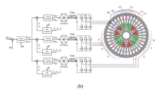
Figure 1.11: Multi-converter system with the same fundamental frequency. a) parallel interleaved converters[67]. b) Triple three-phase machine [76].
