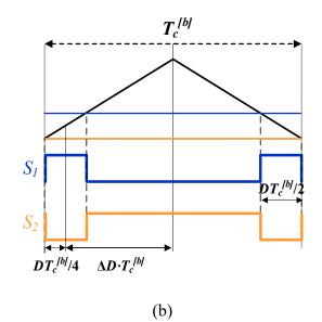
Figure 5.7: EGW operation when the two gate signal pulses of  $S_1$  are going to overlap each other. a)  $\Delta D = D/4$ . b)  $\Delta D = 1/2 - D/4$ .
