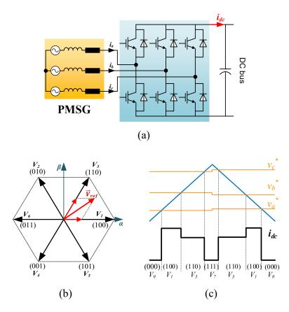
Figure 4.1: Two-level three-phase converter and SVPWM operation. a) Topology, b) Switching vectors and voltage reference, c) Modulation waveform.
