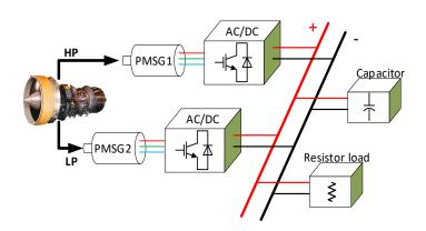
Figure 3.1: Dual-channel enhanced power generation system
