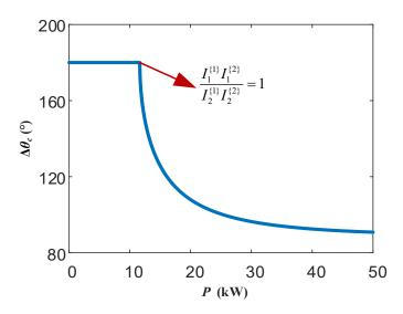
Figure 4.8: Optimised  $\Delta \theta_c$  when power sharing ratio between two converters is 1:1.
