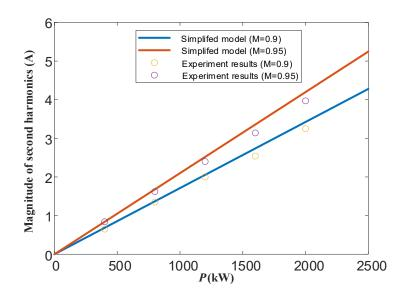
Figure 7.10: Comparison of second carrier harmonic components  $(2f_c)$  between experiment results and simplified model.
