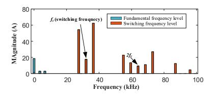
Figure 1.12: Spectrum of DC-side current.
