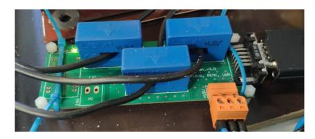
Figure 7.7: Current sensor board.
