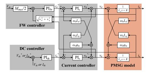
Figure 2.2: Diagram of PMSG system.
