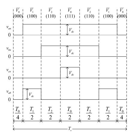
Figure 2.7: Seven-segment switching sequence in Sector I.
