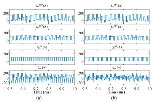
Figure 6.4: Simulation results of  $i_{dc}^{[g1]}$ ,  $i_{dc}^{[g2]}$ ,  $i_{dc}^{[b]}$ ,  $i_{cap}$ . a) Without suppression. b) With suppression.
