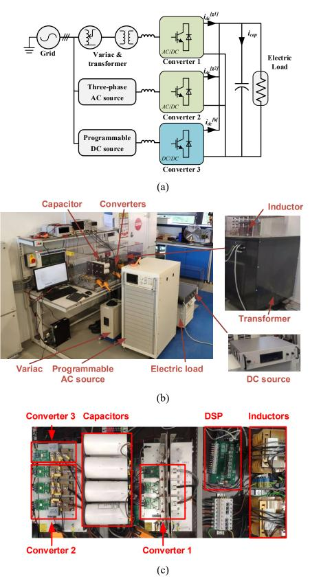
Figure 7.1: Experiment setup. a) Experiment diagram. b) Test rig. c) Converters and the controller.
