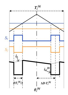
Figure 5.6: Equal-Gate-Width (EGW) PWM
