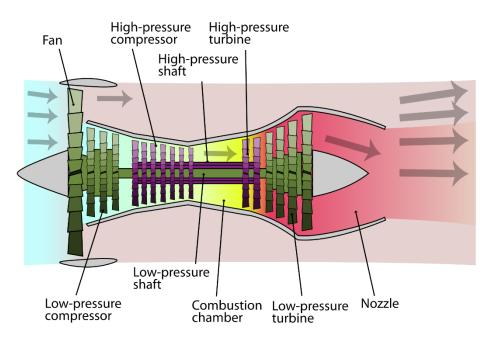
Figure 1.7: Schematic of a twin-spool, high-bypass turbofan engine.
