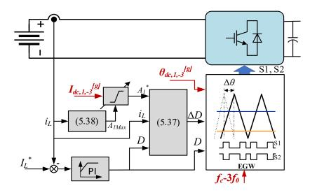
Figure 5.11: Control diagram of battery system.
