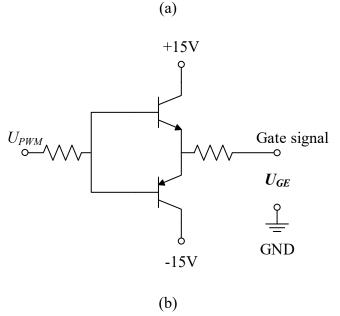
Figure 7.5: Driver board. a) PCB board. b) Push-pull circuit.
