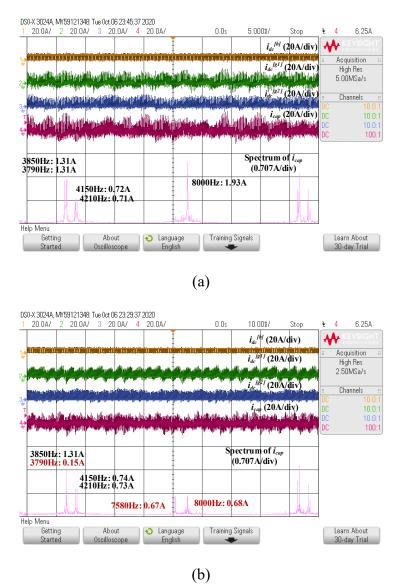
Figure 7.24: Experimental results when  $P^{[b]}=1$ kW,  $P^{[g1]}=1$ kW,  $P^{[g2]}=1$ kW. a) Without optimisation. b) With optimisation.
