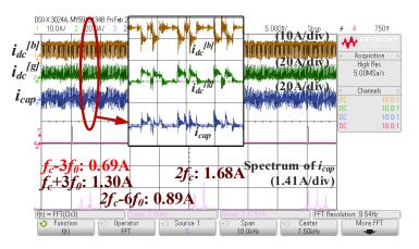
Figure 7.21: Harmonic suppression with EGW suppression when  $P^{[g]}=1$ kW,  $P^{[b]}=1$ kW,  $V_{bat}=180$ V.
