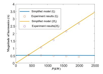
Figure 7.15: Comparison between simplified model and experiment.
