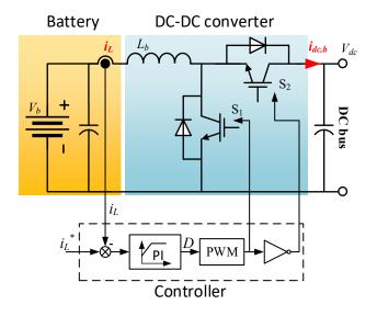
Figure 5.4: Bidirectional buck-boost converter.
