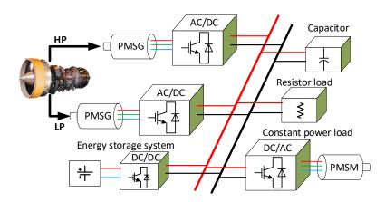
Figure 2.1: Typical dual-generation power system
