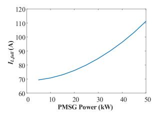
Figure 5.12: *I<sub>L,full</sub>* when the output power of PMSG varies.
