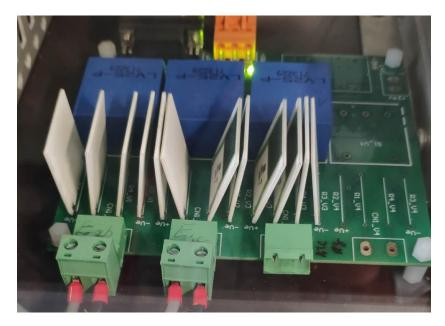
Figure 7.6: Voltage sensor board.
