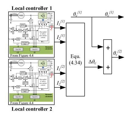
Figure 4.7: Phase-shift controller.
