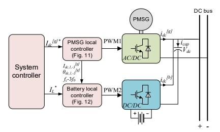
Figure 5.9: Control architecture of the hybrid generation system.
