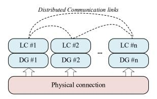
Figure 2.14: Operation principle of distributed control.
