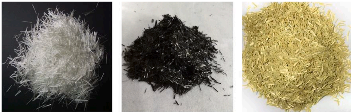
Fig. 1. Chopped glass, carbon and Kevlar fibers with an average grain size of 6 mm.
