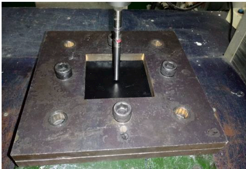
Fig. 2. Dynamic indentation tests using a 10 mm hemispherical indenter and 100*100 mm 2 clamp opening.
