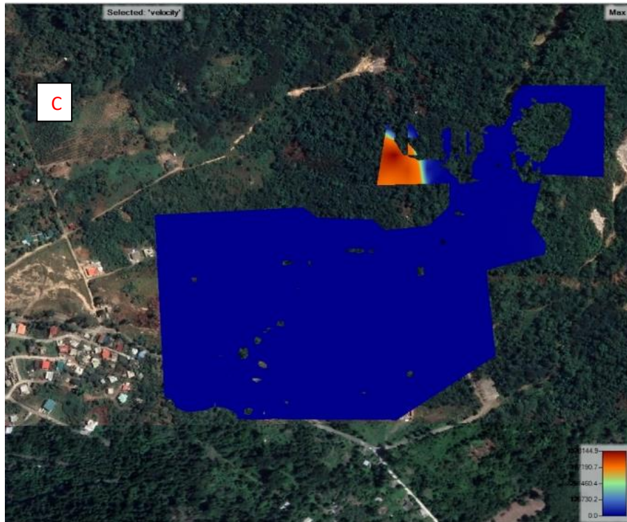
Figure 6.17 C: Results of HEC-RAS unsteady flow simulation for Soufriere (Dominica), showing variations in flow velocity across the floodplain (in m/s).
