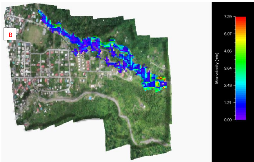
Figure 6.9: RAMMS debris flow simulation of Pointe Michel North (Dominica), (A) Variations in flow height (in m); (B) flow velocity (in m/s) over the whole drainage area.
