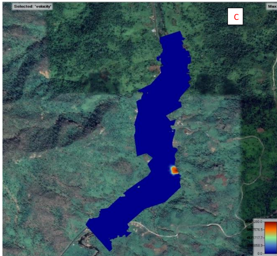
Figure 6.15 C: Results of HEC-RAS unsteady flow simulation for Pagua (Dominica), showing variations in flow velocity across the floodplain (in m/s).
