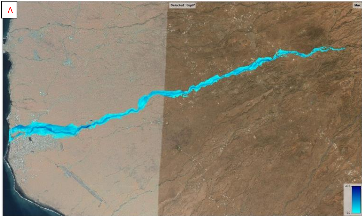
Figure 6.18 A: Results of HEC-RAS unsteady flow simulation for Ribeira Domingo Santo (Fogo), showing variations in flow depth across the floodplain (in m).
