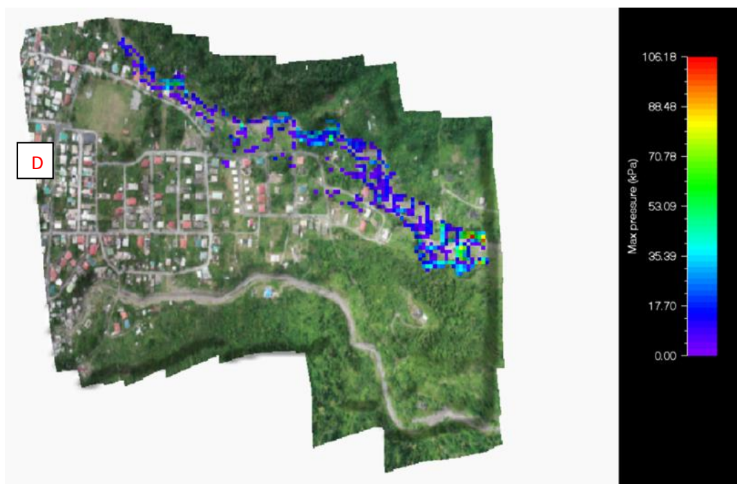
Figure 6.9: RAMMS debris flow simulation of Pointe Michel North (Dominica), (C) flow pressure (in Pa), (D) flow entrainment (in m 3 ) over the whole drainage area.
