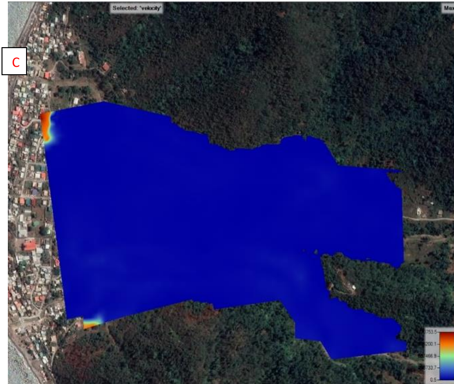
Figure 6.16 C: Results of HEC-RAS unsteady flow simulation for Pointe Michel (Dominica), showing variations in flow velocity across the floodplain (in m/s)
