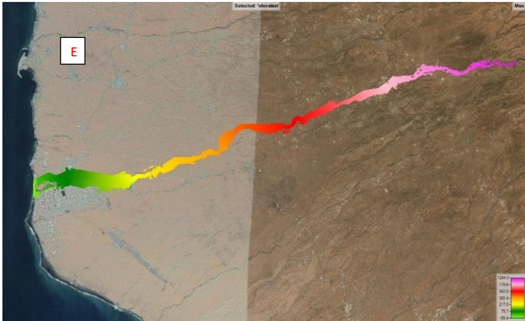
Figure 6.18 E: Results of HEC-RAS unsteady flow simulation for Ribeira Domingo Santo (Fogo), showing variations in water surface elevation across the floodplain (in m).
