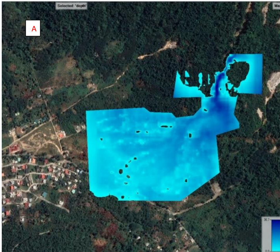
Figure 6.17 A: Results of HEC-RAS unsteady flow simulation for Soufriere (Dominica), showing variations in flow depth across the floodplain (in m).
