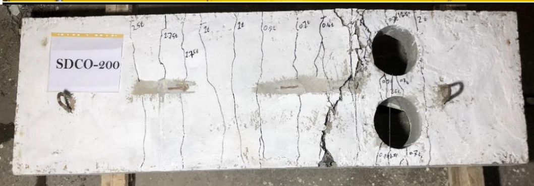
Figure 6. Cracks of SDCO-200 slab.
