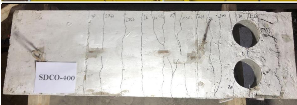
(b) SDCO-400 Slab Top view
