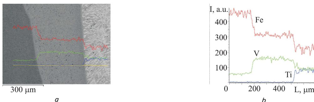
Fig. 14. Transition zone of the Ti-V-Fe junction: a – microstructure; b – distribution of components (electron probe analysis CamScan-4)
