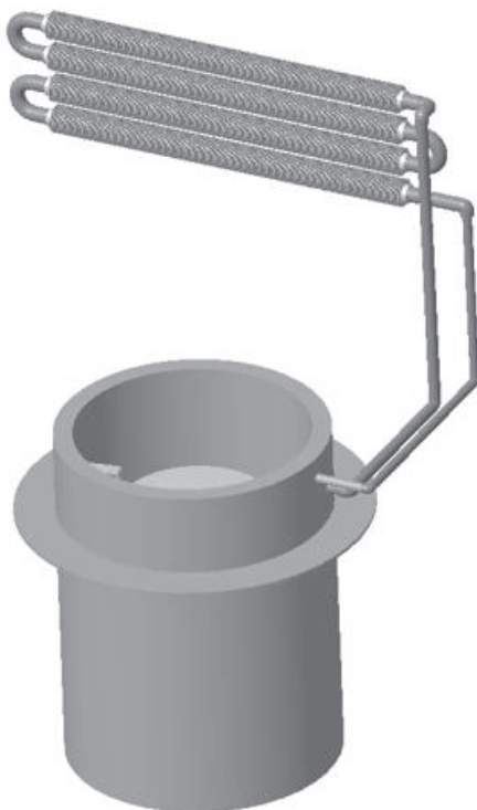
Fig. 6. Condenser and evaporator connection.
