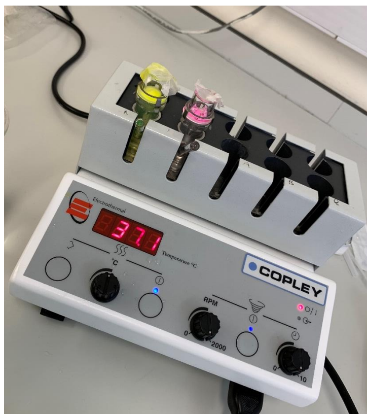
Figure 29: Vertical Franz Diffusion Testing
