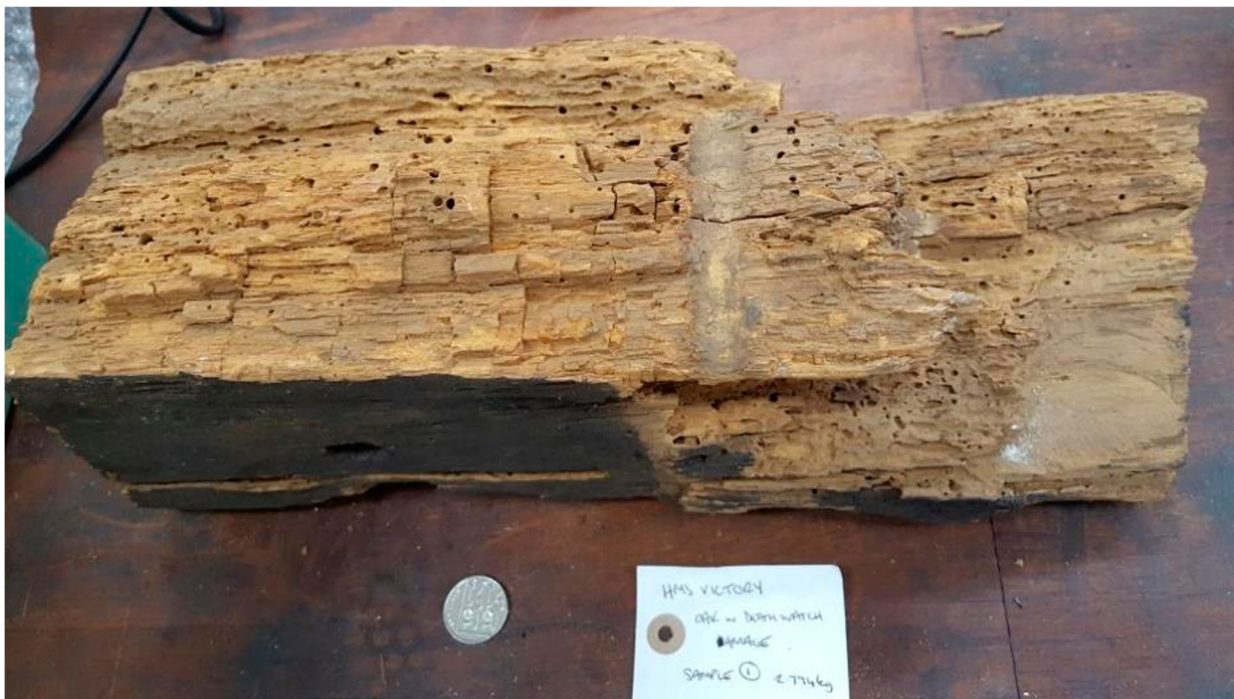
Figure 1. The investigated oak timber (previously removed from Victory ) before subsampling. Note the original, darker and smoother, outer surface. Image taken by R Southwell.
